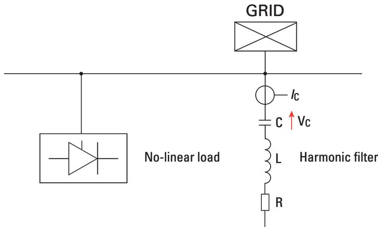
Schematic representation of a filter branch where the voltage across the capacitor is investigated by the peak repetitive overvoltage function - 59H.
