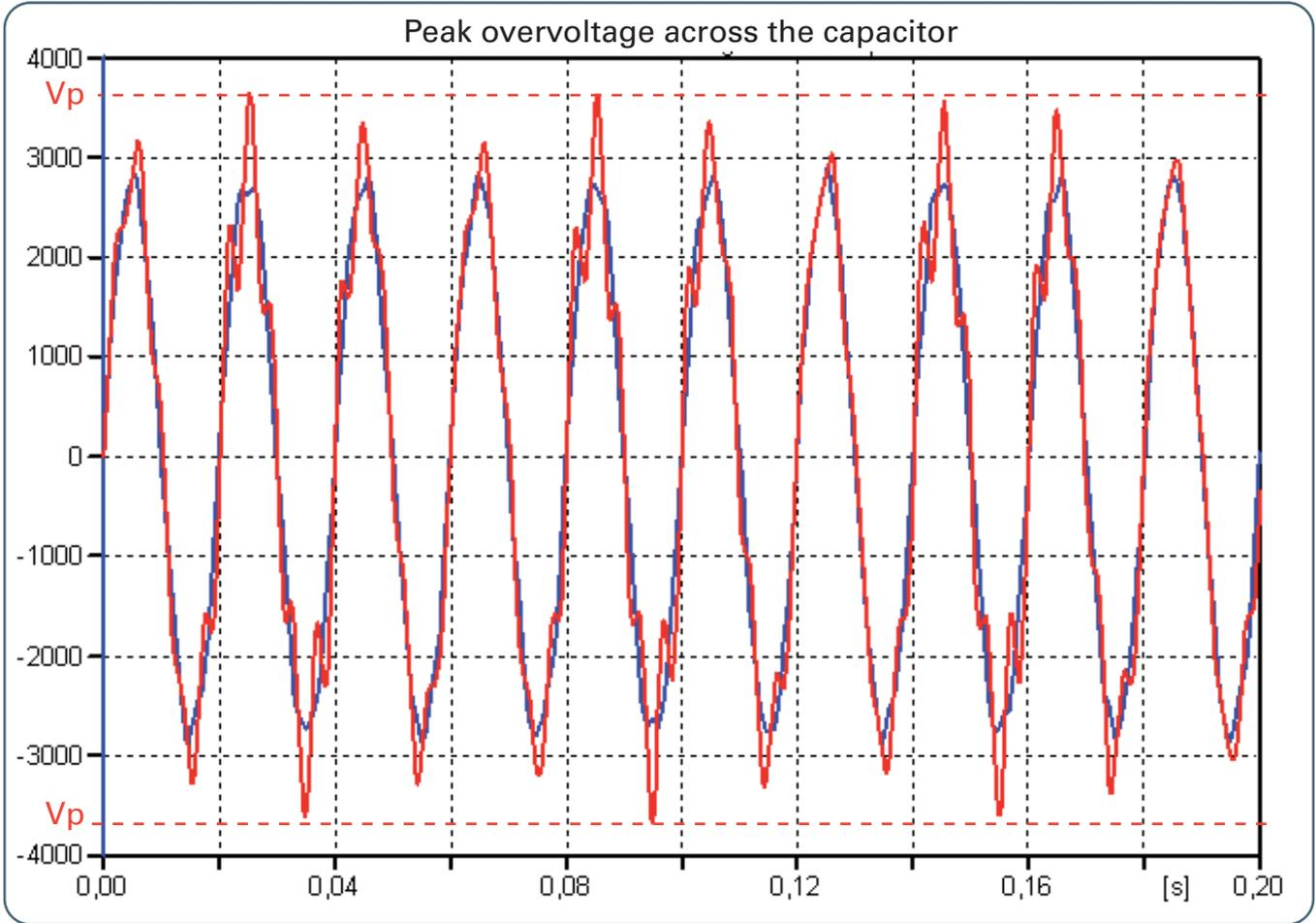
The solution is to calculate the peak repetitive overvoltage (dashed red line), monitored by the 59H function available in NVA100X-C.
