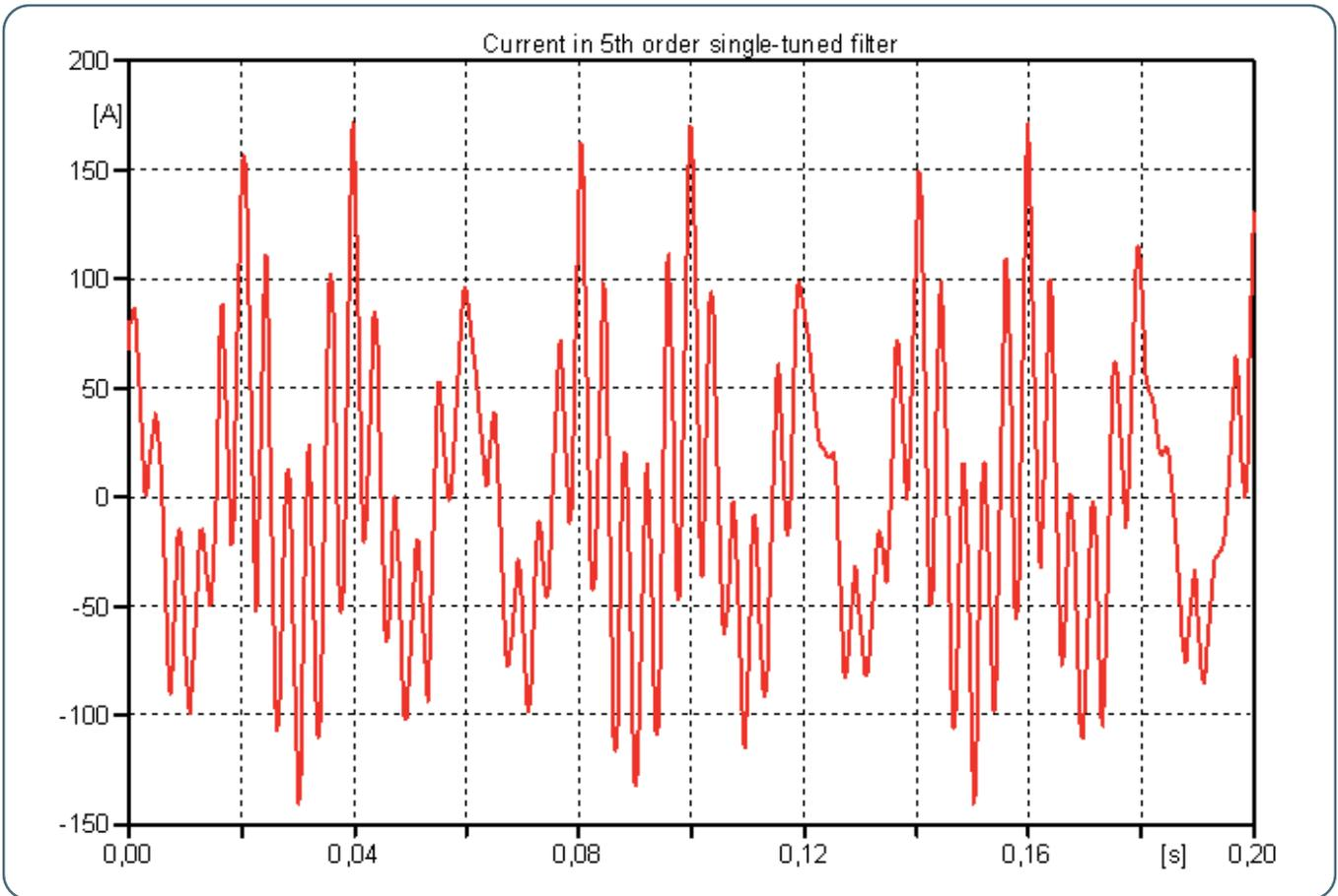
Looking at the electrical quantities into the filter itself they show in detail the real voltage stress at the capacitors; the  $I_{C5}$  current generates the  $V_{C5}$  voltage waveform across the capacitor in the 5th order single-tuned filter
