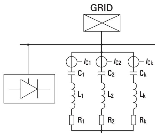
Single-tuned filters - Typical configuration
