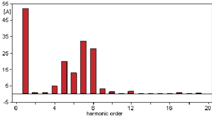
In event of a high harmonic content the 50/51RMS function is requested in a capacitor bank protection. The filter is mainly loaded with the fundamental harmonic and the harmonic to which it is tuned. The analysis of its spectrum shows clearly even the influence of all the other components. The peak of the current of the fundamental component is 52 A while the peak of the true RMS current is around 130 A.
