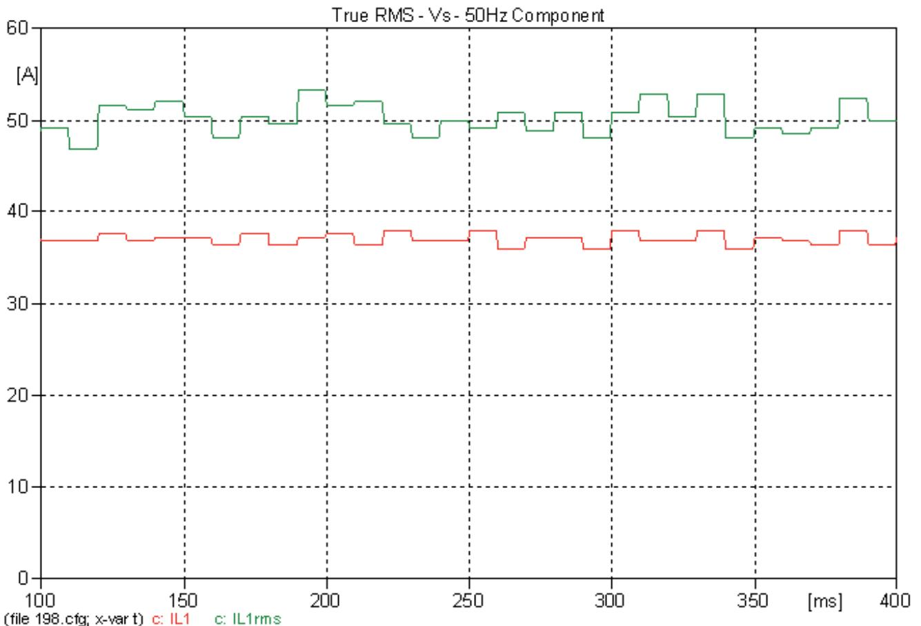
In a protection relay for capacitor bank the availability of the function 50/51RMS phase overcurrent (True RMS type) is requested. The function available in NVA100X-C provide high protection because it realize harmonic analysis up to the 50th order, with three independent thresholds (where the first and second can be set as inverse time curve or definite time).
