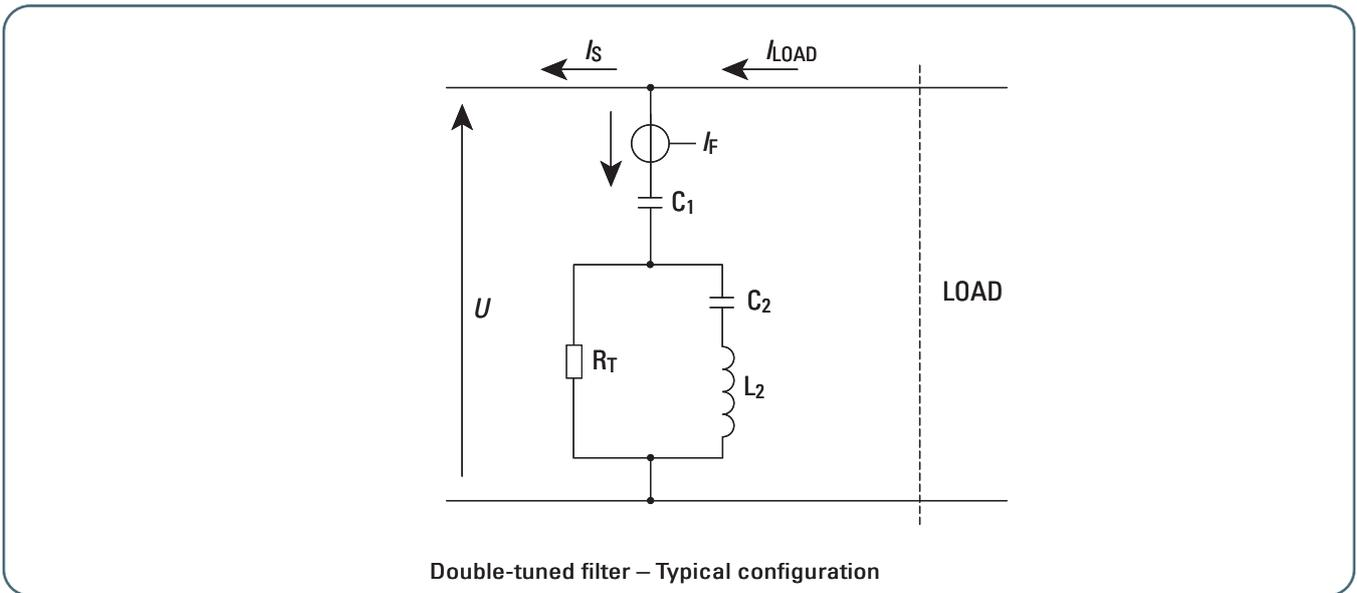
The wide flexibility of NVA100X-C's setup let users also to find a solution for more complex filter configuration such as double-tuned filter and C-type filter (engineers engaged in harmonic filter design can provide a computation about the contributes in terms of harmonic current in each part of the filter).
