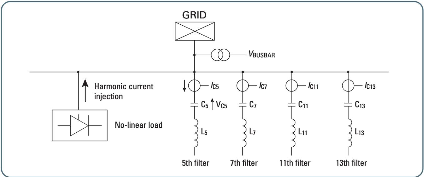
The voltage measured at the MV busbar ( $V_{BUSBAR}$ ) shows an acceptable level of voltage distortion.
