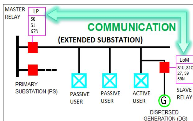
Fig. 2 Communication between PS (master relay) and DG (slave relay).
