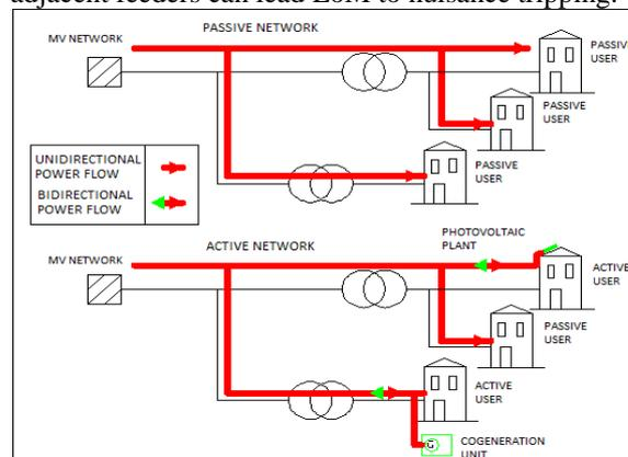
Fig. 1 Power flow on MV network.
